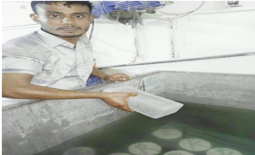
Figure 3.4 Concrete Block Curing
