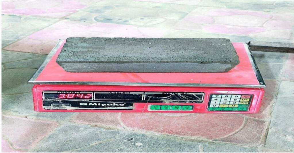
Figure 4.2 Tasted Concrete Block Weight
