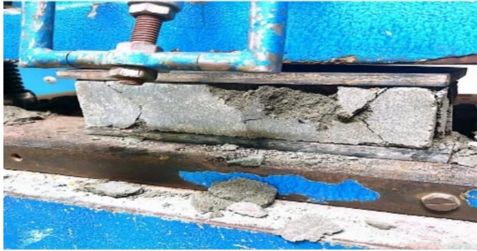
Figure 3.8 Concrete Block Compressive Strength Test
