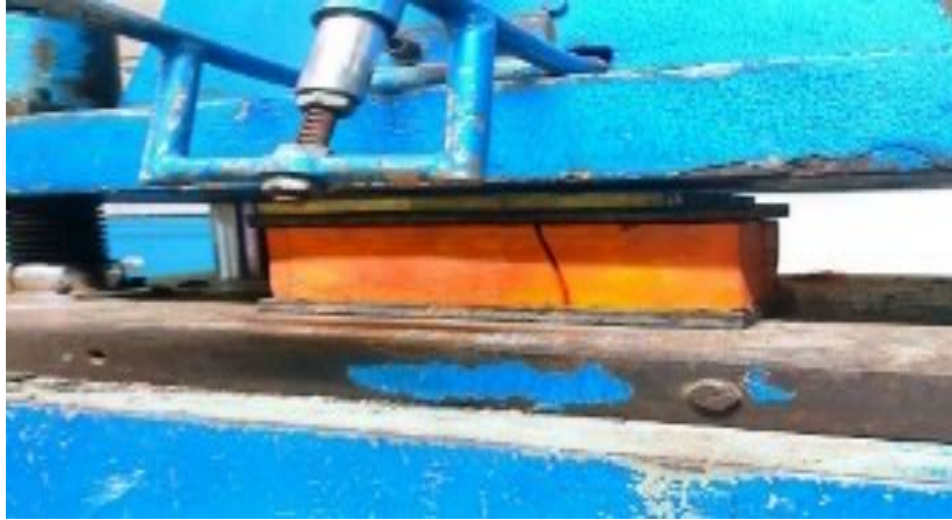
Figure 3 .10 Machine Made Brick Compressive Strength Test
