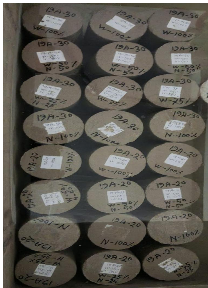
Fig. 3.4: Curing of Cylinder
