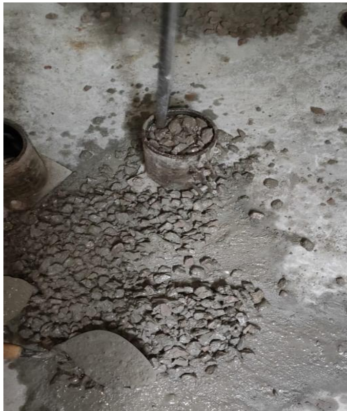
Fig. 3.3: Casting of Cylinder
