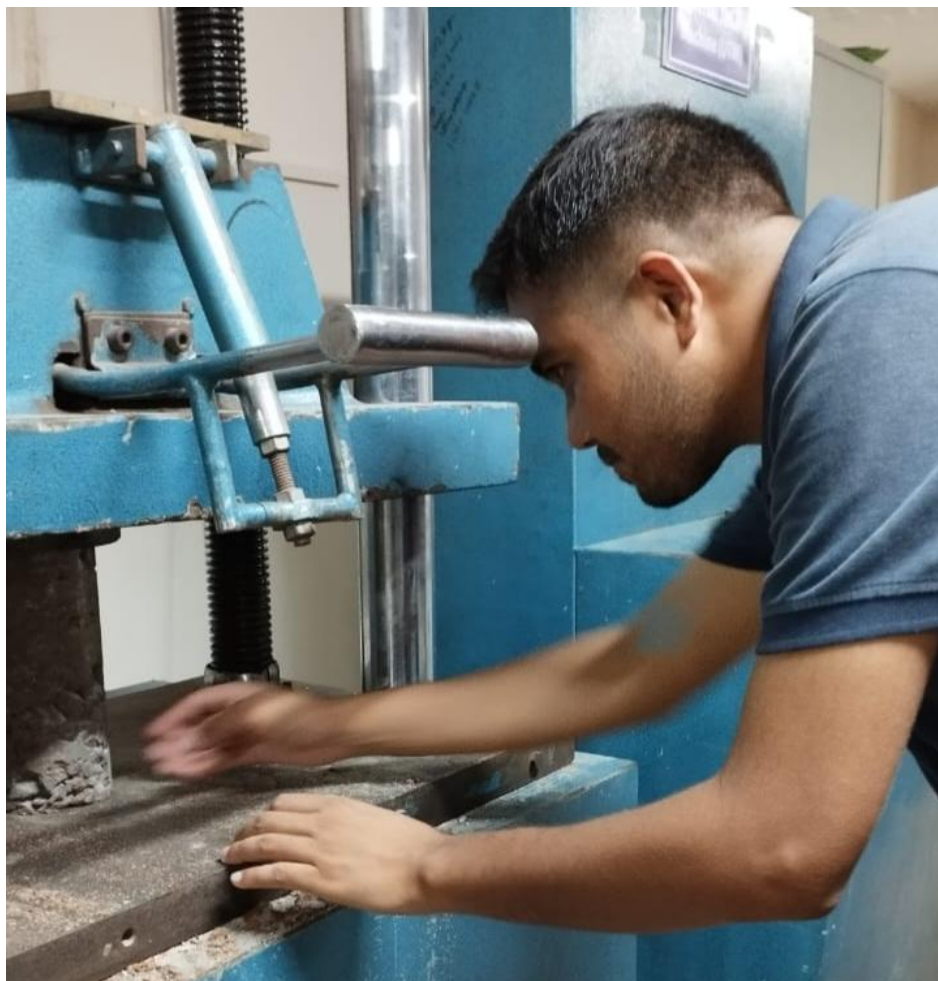
Fig. 3.7: Place the cylinder in UTM machine
