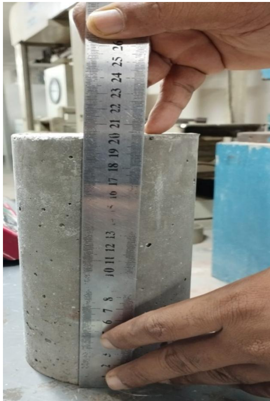
Fig. 3.6: Preparation of Cylinder M15 & M20 measurement Grade
