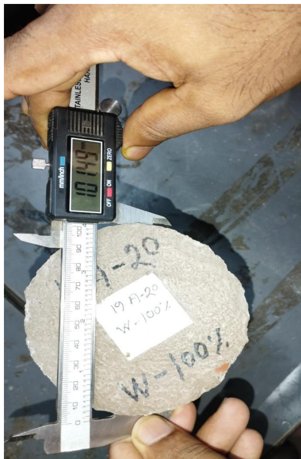
Fig. 3.5: Preparation of Cylinder M15 & M20 Grade
