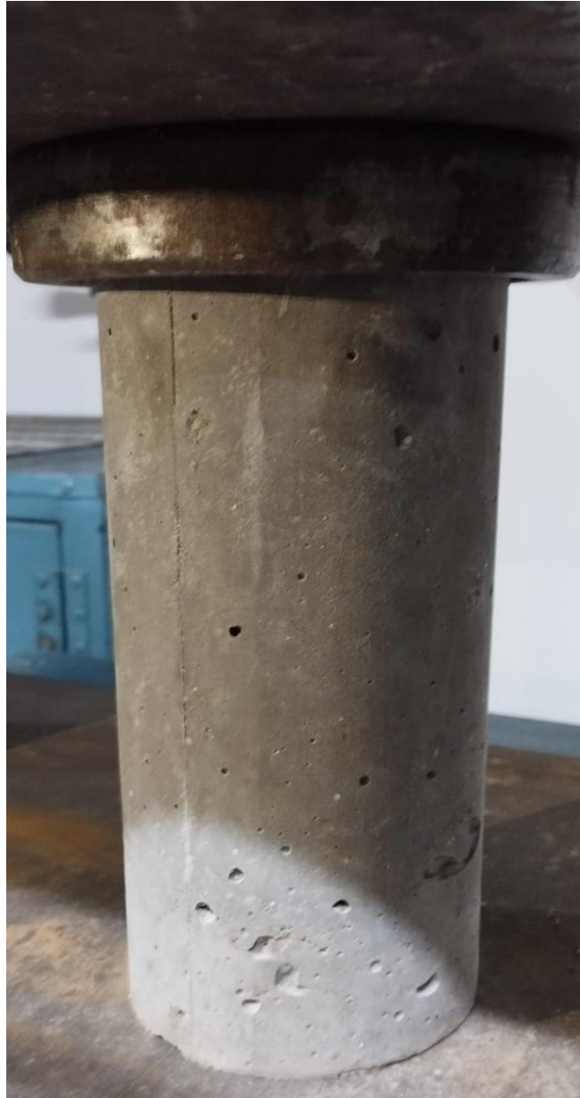
Fig.3.8:Compressive fracture of Cylinder Grade M15 & M20
