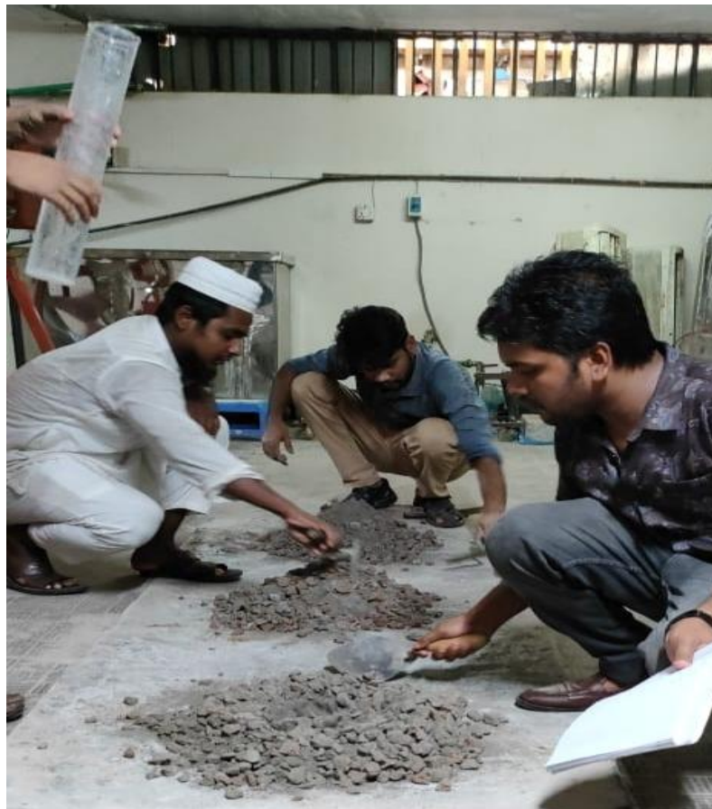
Fig. 3.2: Mixing of Sand Cement and coarse aggregate
