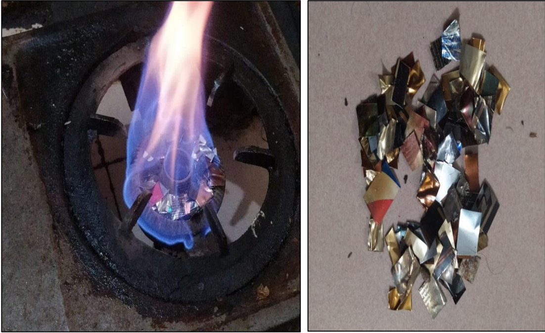
Figure 8: Fire resistance test of drink can
