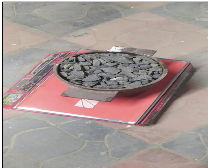
Fig. 6: Unit weight of coarse aggregate
