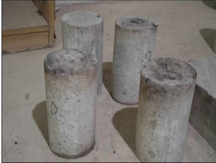
Fig. 3.17: Heating effect of concrete cylinder specimens
