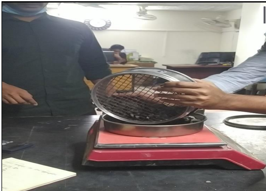
Fig. 2: Sieve analysis of coarse aggregate test
