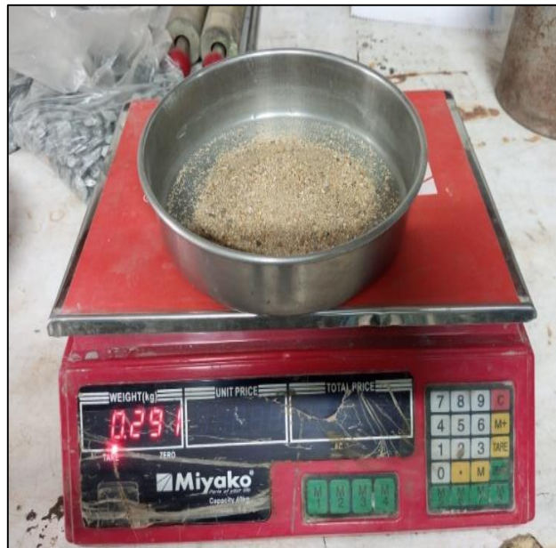
Fig. 3: Specific gravity of fine aggregate test
