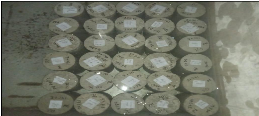
Fig. 3.15: Concrete specimens curing
