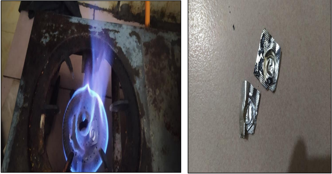
(a) Fire Resistance after first 15 minutes
