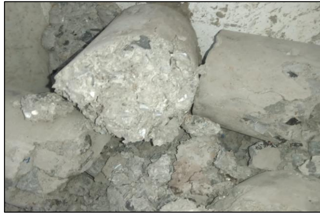
Figure 4.2: Concrete cylinder after compressive strength test
