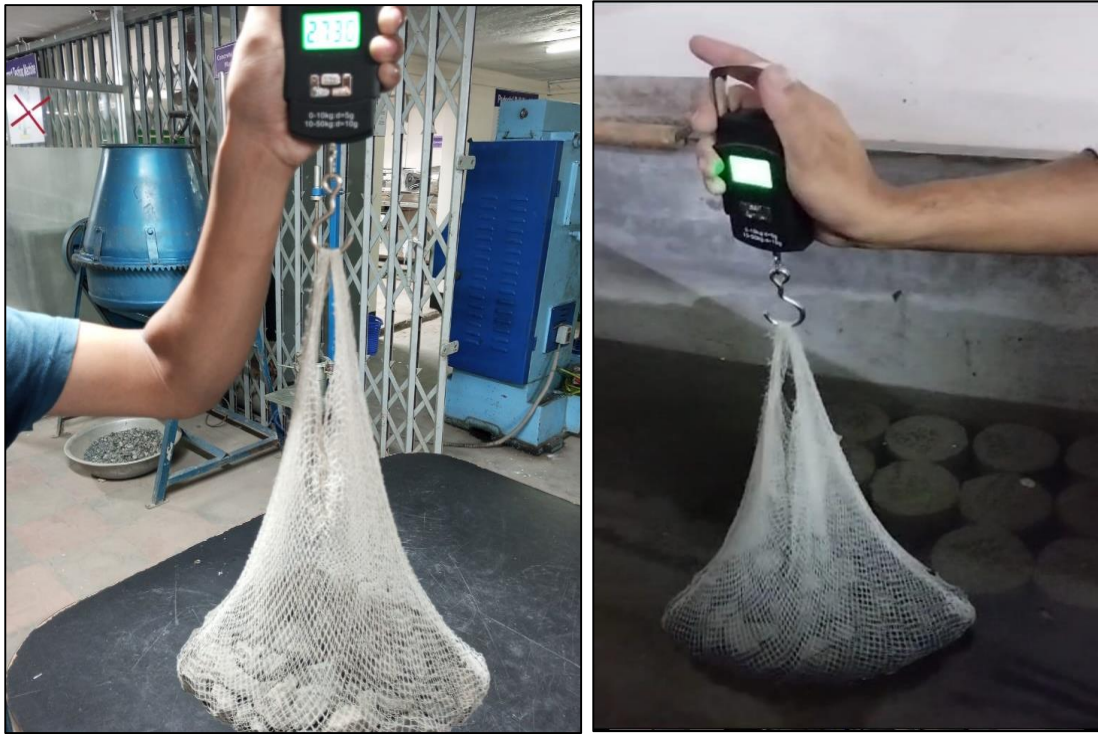
Fig. 4: Specific gravity of coarse aggregate test (Coarse Aggregate weight on air, SSD sample & in water)
