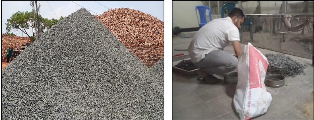
Figure 3.6: Coarse aggregate collect from a stack, clean and separated
