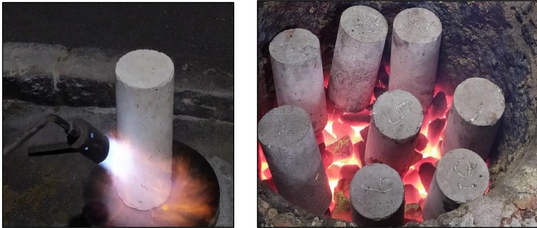
Fig. 3.16: Concrete cylinder specimens heating for temperature balance & deep heating in the oven.
