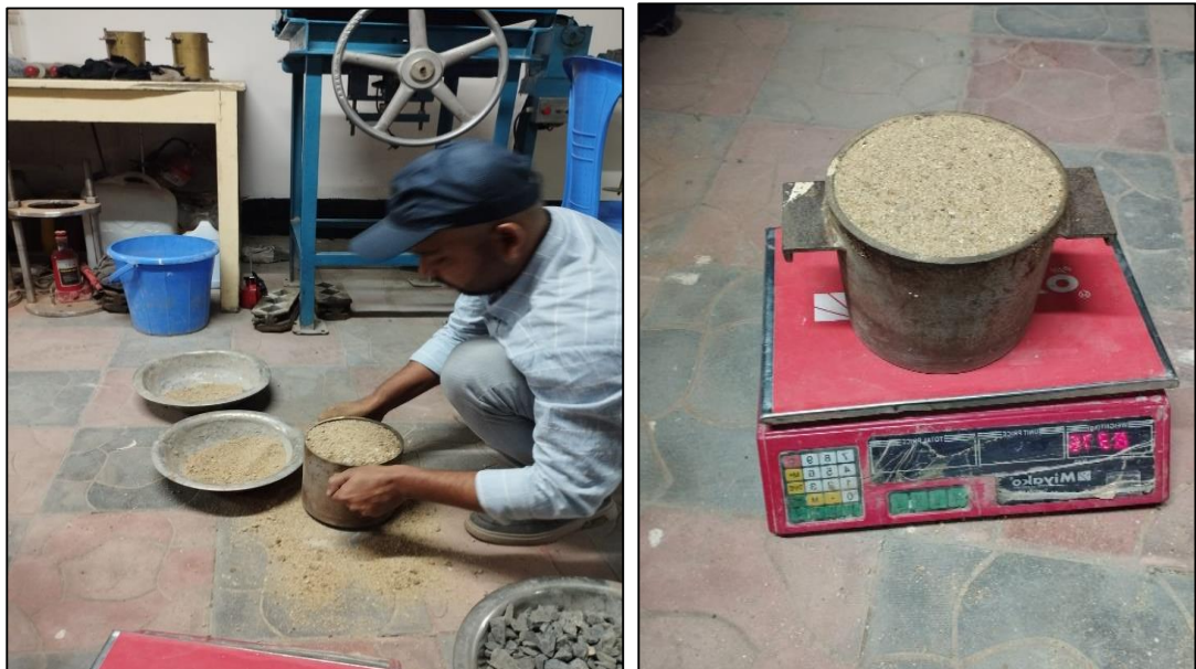
Fig. 5: Unit weight test of fine aggregate
