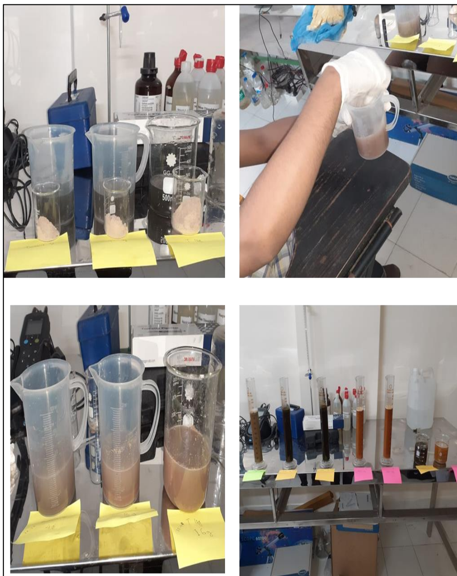
Figure 3.10: Coagulants mixed with wastewater in different dosages.
