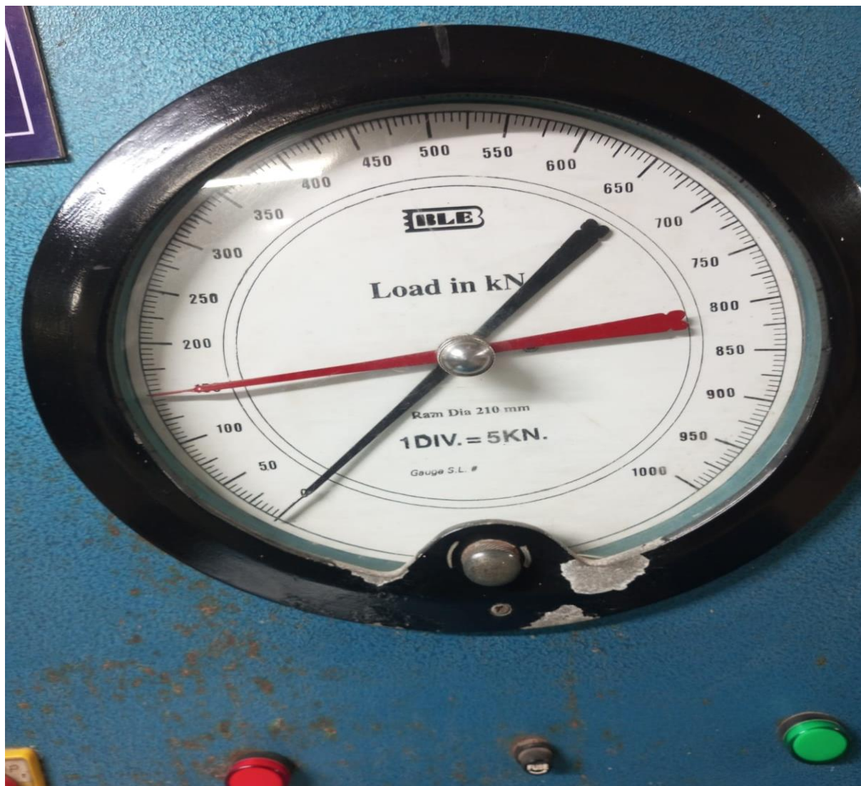
Fig: 4.7.1 Testing compressive strength.
