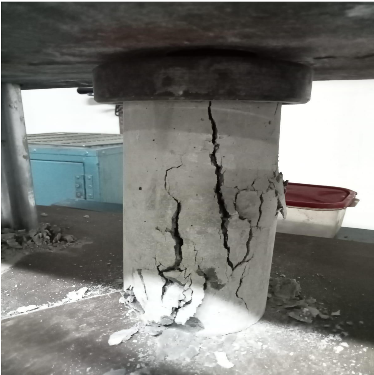
Fig: 4.6.1 Testing compressive strength.
