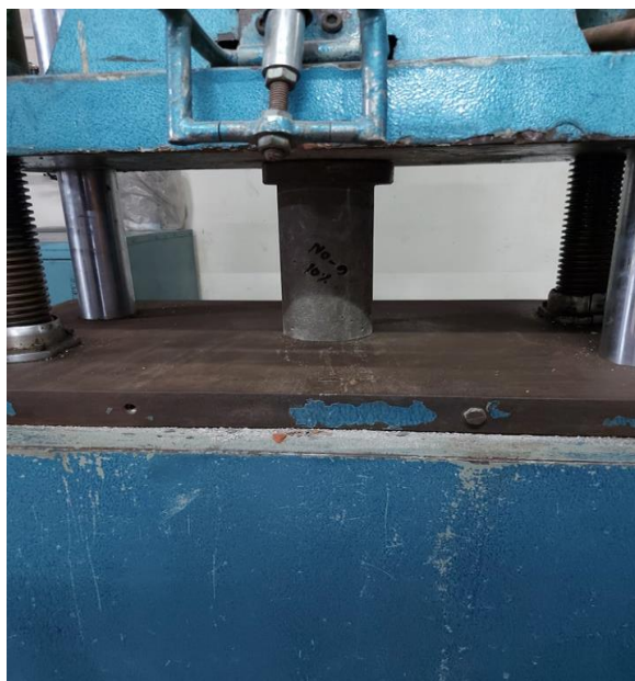
Figure 3.7: Compressive Strength Test
