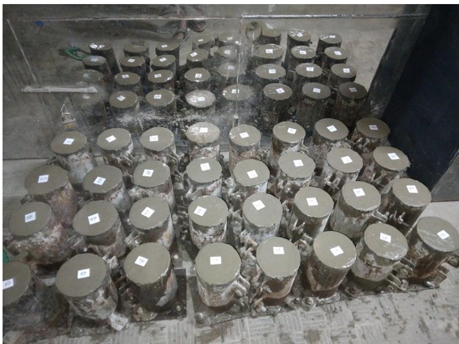
Figure-3.5 Mold of Cylinder.
