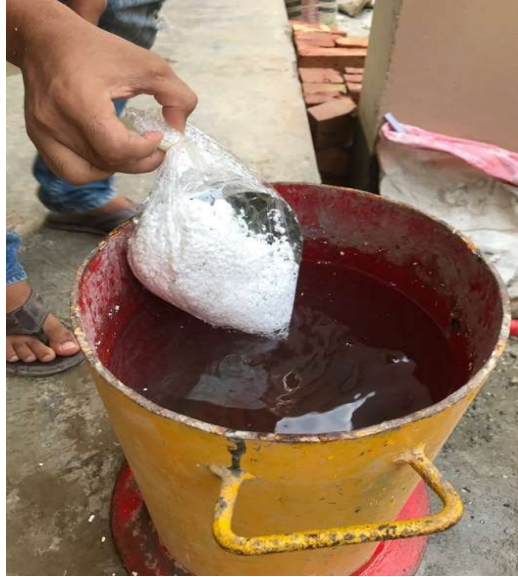
Figure 3.2 Density measurement of EPS beads
