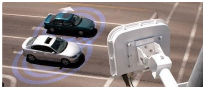
Fig 2.7: Using radar technologies, Smart Sensor HD devices have the capability of detecting vehicles ( Contactless System ).
